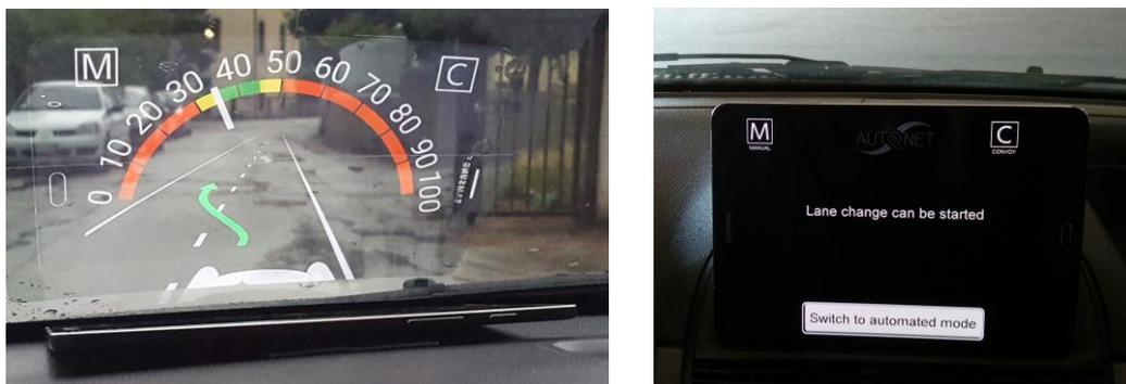
**Figure 8 - AutoNet2030 HUD (left) and secondary device (right) realistic projections**
